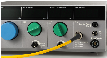
Fiber-optic cable connection to family of OcuLight laser consoles
